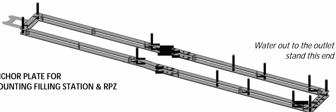
**ANCHOR PLATE FOR MOUNTING FILLING STATION & RPZ**
