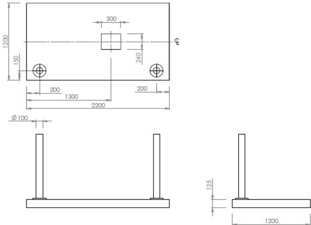
*Note 1: The 300 x 240mm void is **optional**, used to facilitate cable entry and to allow drainage in case of need.*
