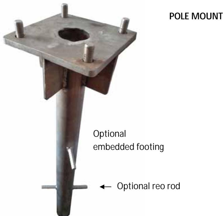
The plate can be embedded flush with the concrete surface or elevated slightly, if this simplifies concreting. If elevated, the gap can be filled with sand cement and parged with a neat 45-degree edging.
