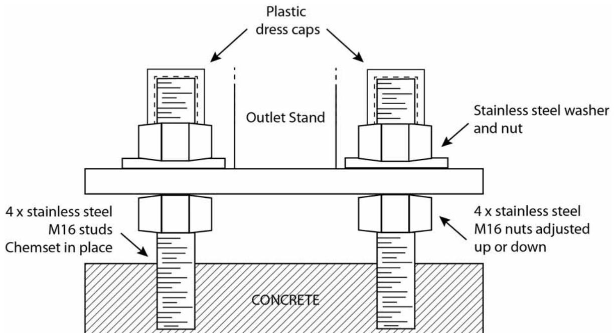
Installation is completed by neatly parging in the underside of the outlet stand with sand and cement, finishing with a smooth 45-degree bevelled edge.
