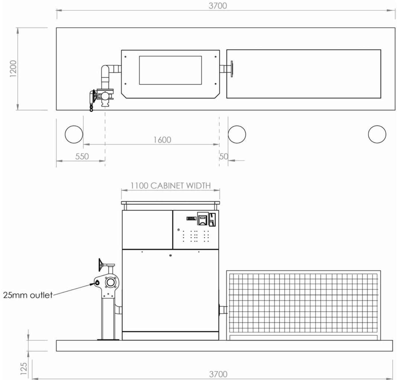
*Note: Right hand entry plumbing shown. Plinth is symmetrical so can be spun 180 degrees to accommodate left hand entry plumbing.*
