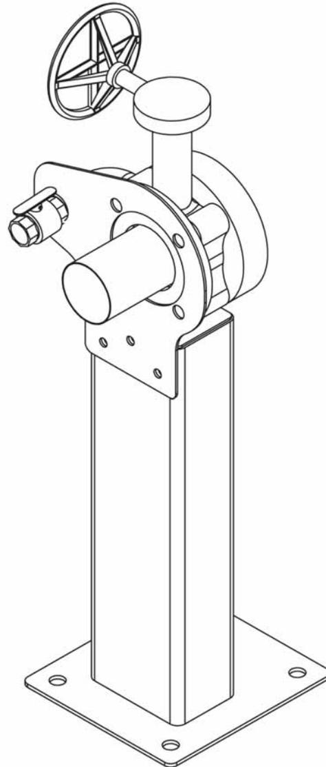
The typical outlets are 80mm and 25mm or 100mm and 25mm. Alternatives are available, example 80mm, 50mm and 25mm.
