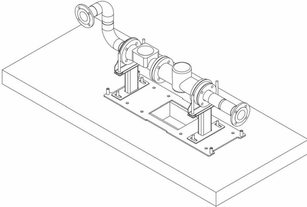
*Note: Slab can be reversed to allow for plumbing to enter from the left hand side. Height of the plumbing can be adjusted by raising or lowering the mounting plates with the M16 nuts on the 4 threaded rods.*
