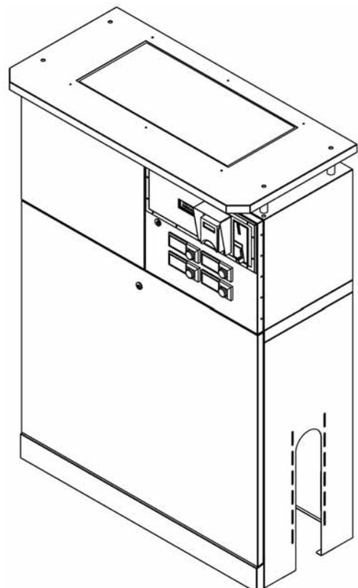
*Note: Cabinet cut outs allow plumbing to enter on either side (right or left). Drawing has the optional cabinet mounted solar panel.*
