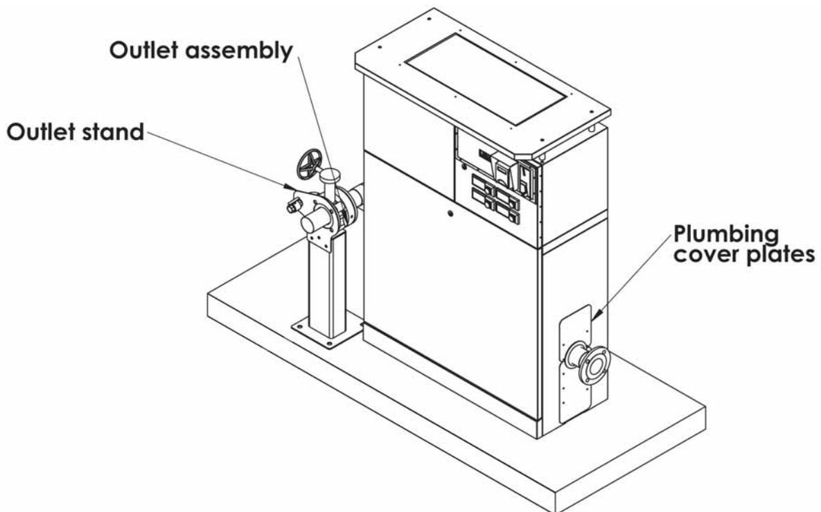
It is normal to have the outlet pointing down slightly to ensure any dirt or contaminant flushes free of the plumbing system. The method of installation is common for 80mm or 100mm systems, although the 100mm tap assembly and stand will mount slightly forward and further away from the cabinet.
