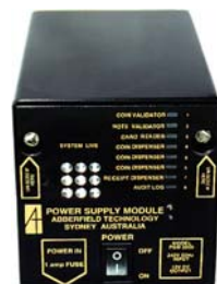
Battery backed power supply
