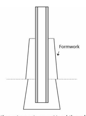
Fitting cast concrete support to existing pole
