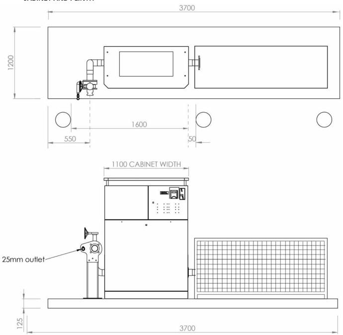
Note: Right hand entry plumbing shown. Plinth is symmetrical so can be spun 180 degrees to accommodate left hand entry plumbing.
