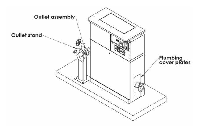
It is normal to have the outlet pointing down slightly to ensure any dirt or contaminant flushes free of the plumbing system. The method of installation is common for 80mm or 100mm systems, although the 100mm tap assembly and stand will mount slightly forward and further away from the cabinet.
