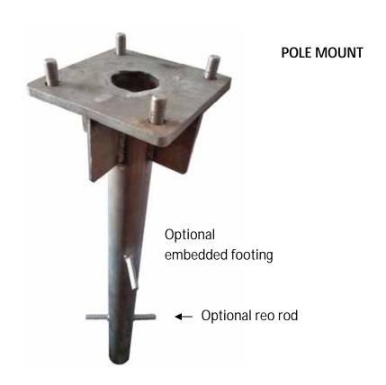
The plate can be embedded flush with the concrete surface or elevated slightly, if this simplifies concreting. If elevated, the gap can be filled with sand cement and parged with a neat 45-degree edging.
