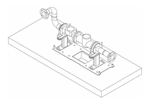
Note: Slab can be reversed to allow for plumbing to enter from the left hand side. Height of the plumbing can be adjusted by raising or lowering the mounting plates with the M16 nuts on the 4 threaded rods.
